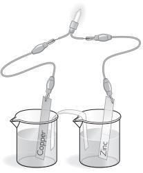
Copper (II) sulfate Zinc sulfate
